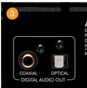
1 The CD17 remote offers system control of matching Arcam products. 2 Dual line outputs allow for connection to multi-room systems. 3 Digital outputs allow for future upgrading, e.g. with a D33 DAC.
